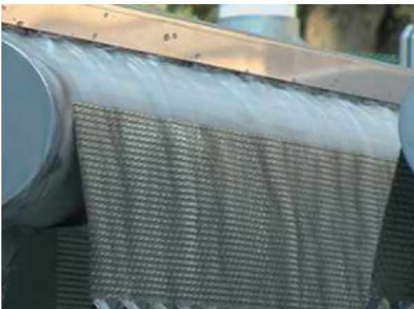
Aspect of flowing down liquid from a diffuser panel.
