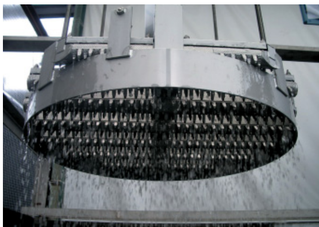
Aspect of flowing down liquid from a diffuser panel.
